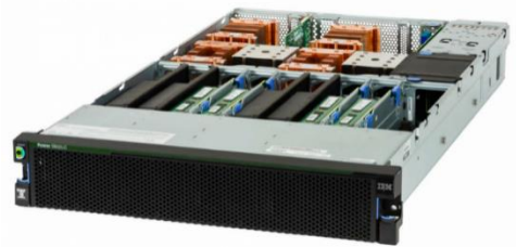
2 x P8 Minsky with NVLink GPUs
