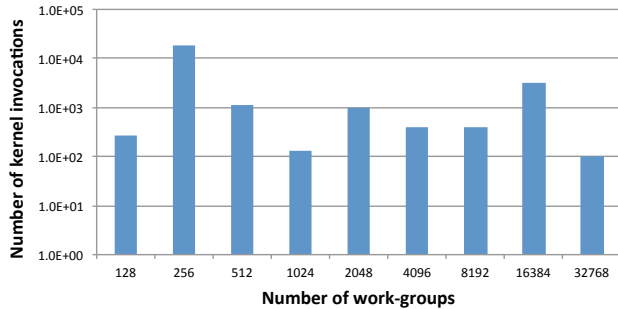
Figure 2. Distribution of number of work-groups among kernel launches in Parboil and Rodinia benchmarks
