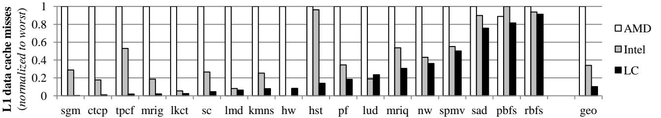
Figure 8: Locality comparison of AMD, Intel, and LC compilation approaches. Results are normalized to the worst performing tool. LC has geomean reduction in L1 data cache misses of  $9.81 \times$  and  $3.35 \times$  over AMD and Intel respectively.
