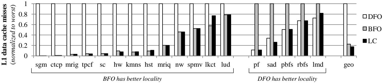
Figure 7: Locality comparison of DFO, BFO, and locality-centric (LC) scheduling. Results are normalized to the worst performing schedule. LC has geomean reduction in L1 data cache misses of  $5.72 \times$  and  $1.29 \times$  over DFO and BFO respectively.
