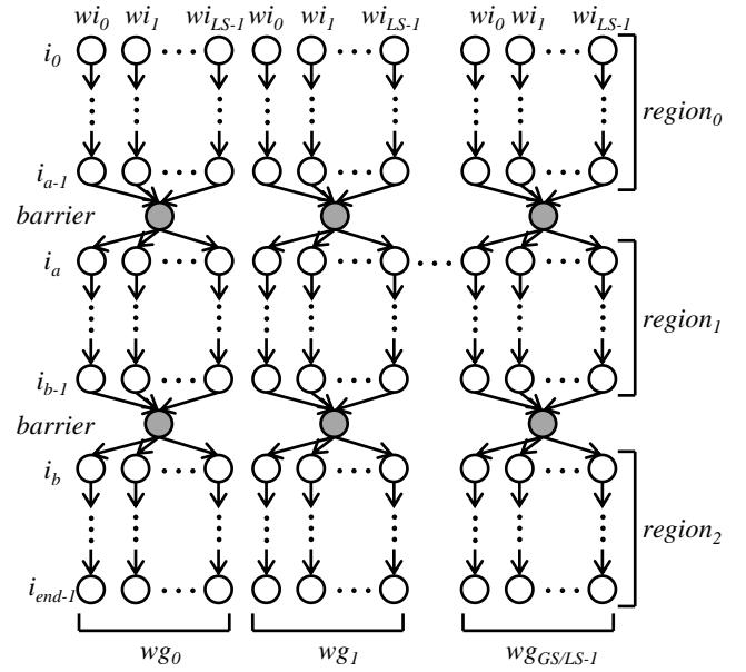
Figure 1: Immediate dependencies between dynamic instructions or instruction blocks ( $i$ ) in OpenCL kernels. Each work-group ( $wg$ ) contains local size (LS) work-items ( $wi$ ). Work-items in different work-groups execute independently until completion. Work-items in the same work group synchronize at barriers. Barriers divide the program into code regions within which work-items execute independently. Work-item independence within regions provides great flexibility for work-item scheduling.
