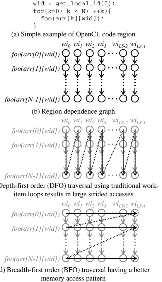
Figure 2: A motivating example demonstrating the impact of scheduling on the memory access pattern.
