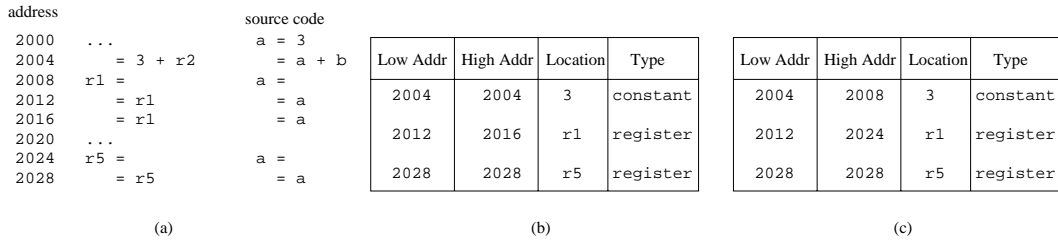
Figure 1: (a) An example code segment (b) range records for variable a (c) extended range records for variable a
