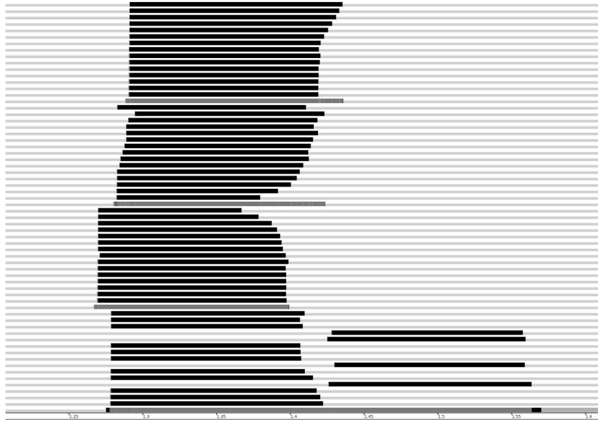
Figure 6.8: An execution trace of sgemm on four cluster nodes as displayed by the Eden trace viewer. Each horizontal band is a core’s execution timeline. Wide black bars indicate computation, wide grey bars indicated blocked or delayed execution, and narrow light bars indicate idling. The four bars displaced to the right show that four processors started late.
