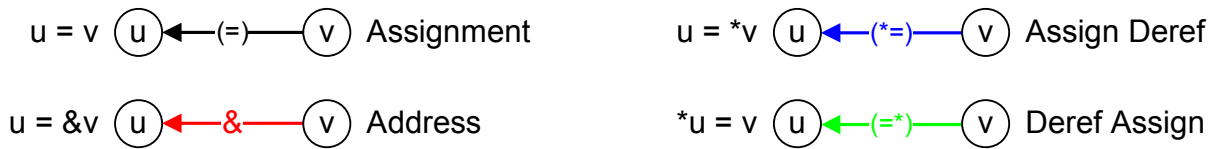
Figure 2.3 Constraint graph grammar where \& specifies the address operator and * is the dereference operator. These four relations are sufficient to describe all assignment relations in the absence of field sensitivity.
