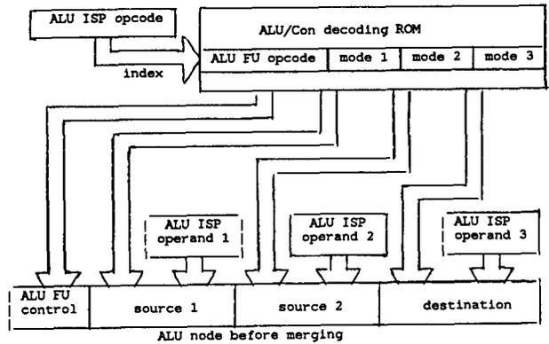
Figure 4. ALU Operation Decoding
