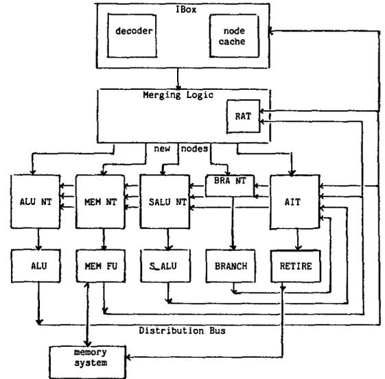
Figure 2. HPSm Data Path
