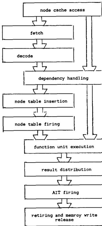
Figure 3. Pipelined View of HPSm
