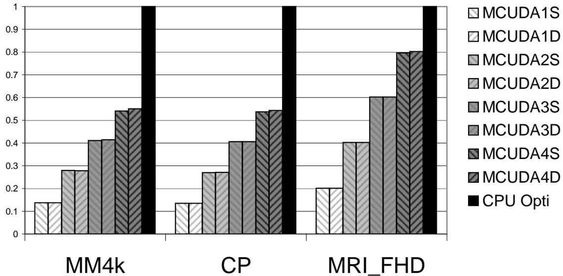
Figure 6: Performance (inverse runtime) of MCUDA kernels relative to optimized CPU code. MCUDA results vary by the number of worker threads (1-4) and the use of (S)tatic or (D)ynamic block scheduling. CPU Opti implementations are parallelized across 4 threads.
