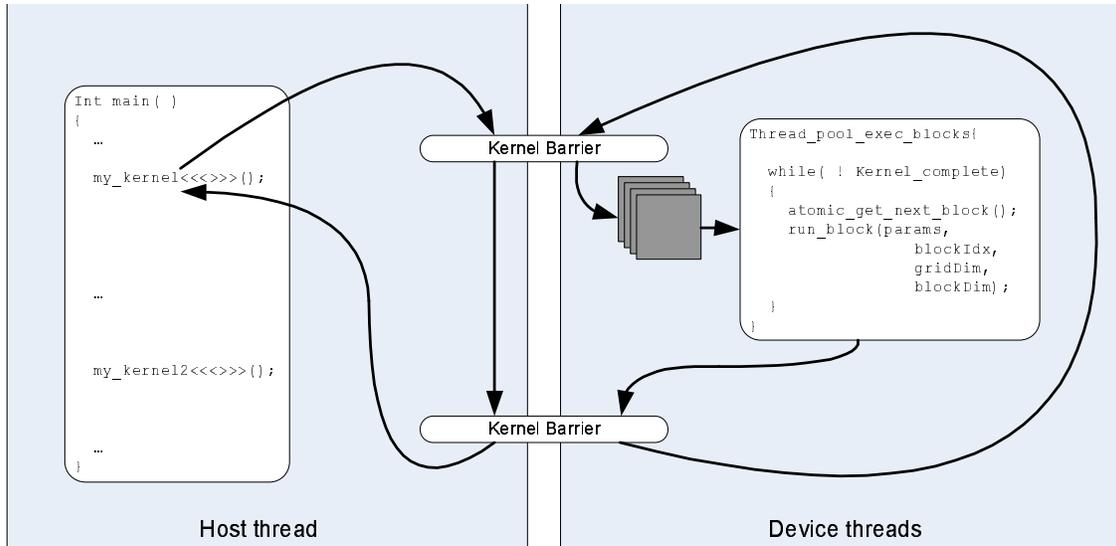
Figure 5: MCUDA runtime framework using dynamic block assignment
