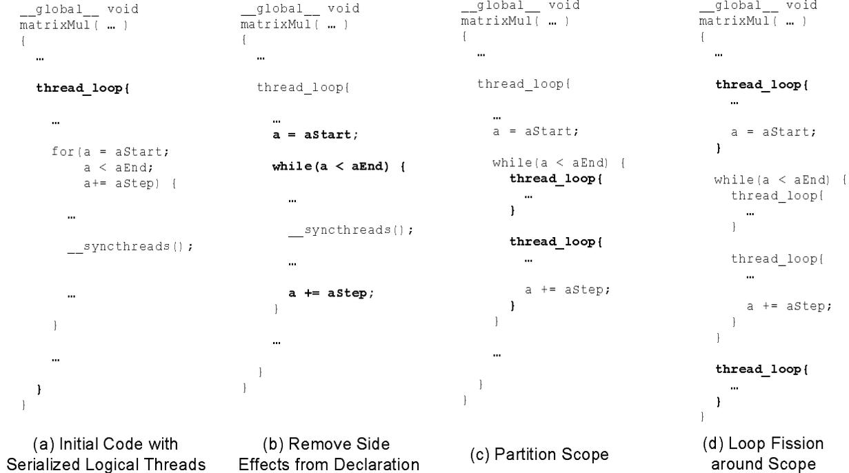
Figure 2: Applying deep fission in Matrix Multiplication to enforce synchronization.
