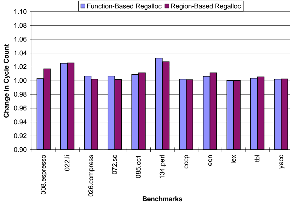
Figure 6.13 Comparison of function-based and region-based cycle count after register allocation of superblock ILP optimized code on a four-issue processor.
