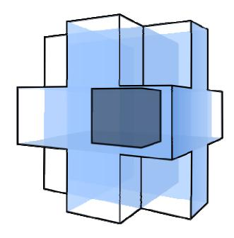
Flow through a cell (dark blue) is updated based on its flow and the flow in 18 neighboring cells (light blue).
